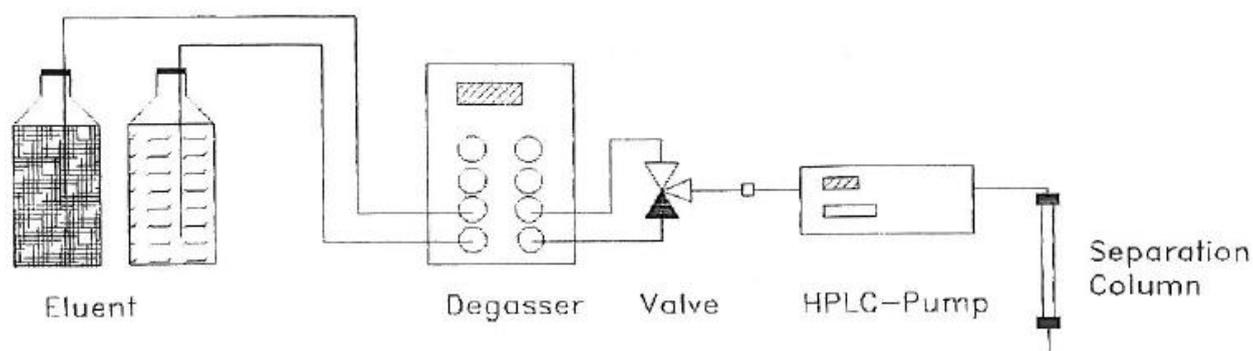
**Fig. 2: Flow diagram of a low-pressure system with installed degasser**
