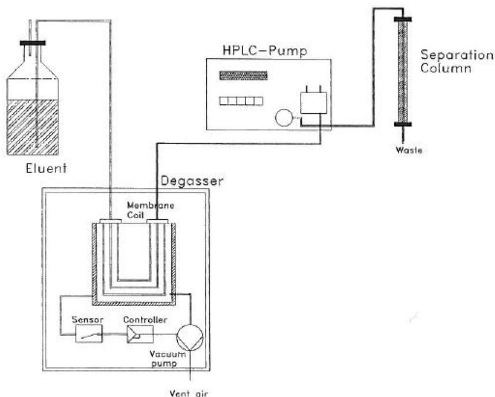
**Fig. 1** The vacuum pump is controlled with a pressure switch, so a vacuum is constantly applied (between approx. -850 up to approx. -890 mbar).
