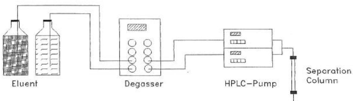
**Fig. 3: Flow diagram of a high-pressure system**
