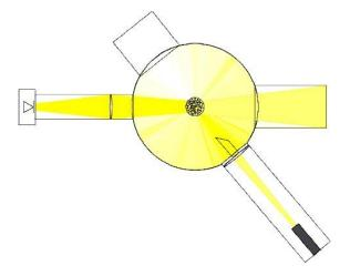
The small particles will cause scattered radiation which is detected using a photomultiplier. The angel between light source and photomultiplier is 120°.
