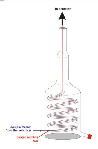
The evaporation chamber is also made of glass, resulting in an easy to clean part of the detector. The flow of the additional gas stream is controlled by a mass flow controller. Gas flow and gas temperature can be adjusted by the user. By adjusting these parameters the detection can be optimized depending on the analytical problem.
