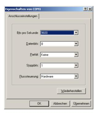
Click the <OK> button to establish the communication with the ZAM3000 detector. The terminal window will be show on your screen like the following example.
