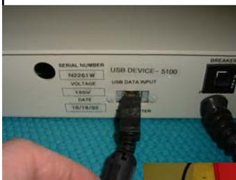
**On a GC the device I.D.# is printed next to the USB jack on the side on the instrument.**
