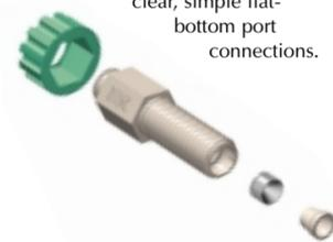
The 1/8" TF fitting has its compression ring preinstalled in the proper orientation so you save time plumbing the valve. The unique 1/16" TF fitting uses an all PEEK design where the parts snap together and function as a one-piece flat-bottom fitting. With higher pressure capability than a standard flangeless fitting and ChromTRAC compatibility, RheFlex TF fittings provide an ideal solution for a variety of applications.
