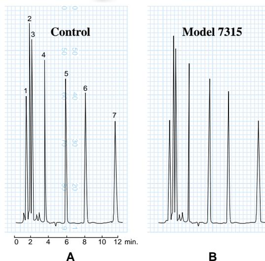
**Fig. 1. Chromatograms from micro-scale HPLC systems. The control system "A" contains a 1 mm x 300 mm microbore column (with 4 µm packing) connected to the injector by a 0.13 mm ID x 60 mm connecting tube with no filter. The other system "B" contains Model 7315 Column Inlet Filter connected between the injector and the microbore column using two connecting tubes.**
