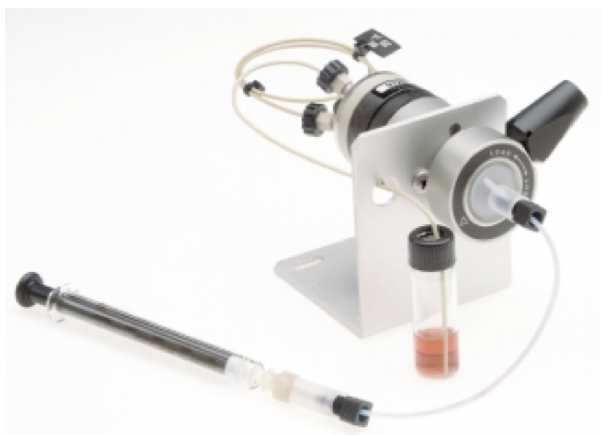
Figure 6. Sample loading by suction through a dip tube. A Model 7252 2.5 mL syringe is shown connected to the valve needle port using a Model 9125-076 Needle Port Adapter.
